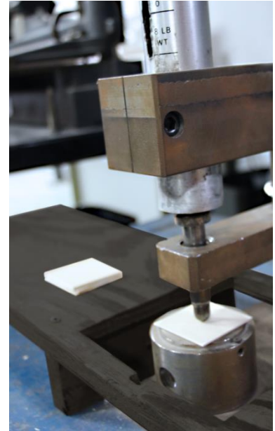
At top: Falling weight drop dart test with GE geometry: the smallest outer diameter and largest rounded metal head. At bottom: Geometries for HIC zones are stronger than ever. KYDEX ® 6523HI compared to non-HIC sheet results from Gardner Drop Dart Impact Testing.
