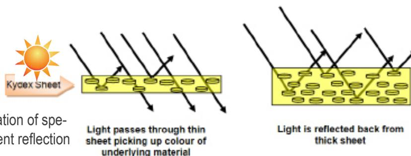
Figure 3: Illustration of special effect pigment reflection and opacity
