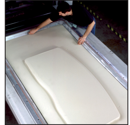
Kiva table top of KYDEX® sheet laminated to MDF core exits Thermolaminator membrane press at H & R Wood Specialties.
